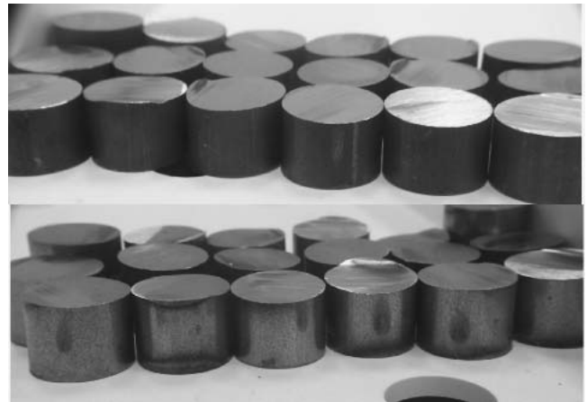
Fig. 3 Samples used for experiment. The upper samples are the non-cold drawn (as rolled), while the lower ones are the cold-drawn materials.
